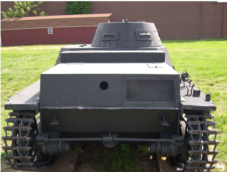
Panzer I (GERMANY): Tank. Produced: 1934-1938. Crew: 2. Main Armament: -. Machineguns: 2. Max Armor: 12 mm. Horsepower: 57 hp. Weight: 5.5 tons. Max Speed: 22 mph. Range: 125 miles. Qty. Produced: 2,000. Pros: Allowed the Germans to practice operating tanks. Cons: Too light for WWII combat. Notes: This tank was designed for training rather than real combat. Nonetheless, it saw extensive service in the battles for Poland, France and elsewhere. Its quick speed allowed it to help create havoc and confusion once it penetrated enemy lines. This vehicle was photographed at Aberdeen Proving Ground, Maryland.
