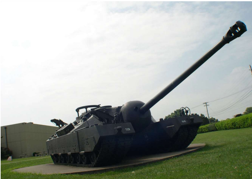
T28 (UNITED STATES): Late WWII Tank Destroyer. Crew: 8. Main Armament: 105 mm. Machineguns: 1. Max. Armor: 25-300 mm. Horsepower: 410 hp. Weight: 95 tons. Max Speed: 8 mph. Range: 100 miles. Number Produced: 2. Pros: Tremendous main gun and armor. Cons: Incredible weight. No turret. Notes: The T28 mounted a very powerful 105 mm anti-tank gun in a fixed superstructure. But instead of just one pair of tracks, the T28 had two tracks per side to handle the vehicle's massive weight. The outer tracks could be removed to allow the T28 to pass more easily in places and for easier transport. The dismantled tracks could be paired to each other and then towed by the T28 or by another vehicle. Only two were ever built; neither made it to combat, and one burned up in a fire.
