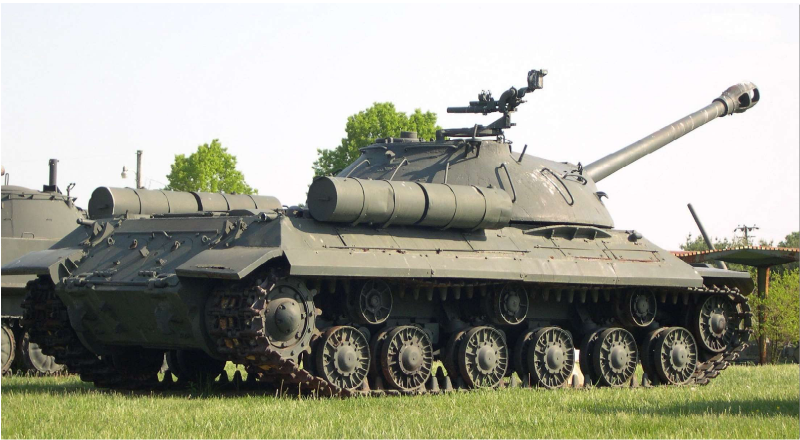
IS-3 (USSR): Late WWII Tank. Crew: 4. Main Armament: 122 mm. Machineguns: 2. Max. Armor: 230 mm. Horsepower: 600 hp. Weight: 46.5 tons. Max Speed: 23 mph. Range: 192 miles. Number Produced: 2,311. Pros: The overall best combination of armor, gun and speed of any tank in the war. Cons: Appeared too late to fight. Notes: The IS-3 was WWII's ultimate progression of the KV tank (KV-1, KV-1S, KV-85, IS-1, IS-2 and IS-3). It was named after Joseph Stalin (Iosef Stalin in Russian), hence the frequent usage of JS-1, JS-2, and JS-3 for the series in English. The shape of its "inverted frying pan" turret was revolutionary and influenced so many of the post-war tanks.
