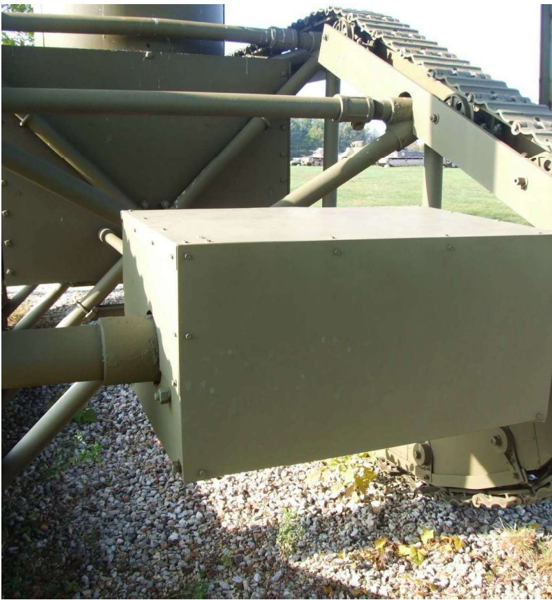
Skelton (UNITED STATES): Late WWI Tank. Crew: 2. Main Armament: 0. Machineguns: 1. Max. Armor: 13 mm. Horsepower: 100 hp. Weight: 9 tons. Max Speed: 5 mph. Range: 34 miles. Number Produced: 1. Pros: Light weight, long track for crossing wide trenches. Smaller target than other large tanks. Cons: Crew and engine in the small box compartment. Notes: This prototype is another example of American attempts to produce a decent tank. Its rhomboid track echoed that of the British heavy tanks, but the crew and engine compartment was a box suspended in the middle. This approach would have permitted the two man crew to cross large trenches to advance a machinegun closer to the enemy. But since the compartment wasn't large enough for larger weapons, the Skelton was never put into production.
