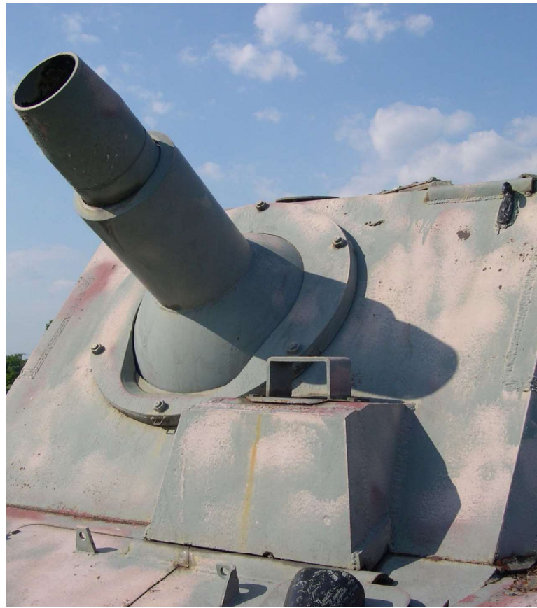
Sturmpanzers IV Brummbär (GERMANY): Mid-WWII Self Propelled Gun. Crew: 5. Main Armament: 150 mm. Machineguns: 1. Max Armor: 100 mm. Horsepower: 296 hp. Weight: 28.2 tons. Max Speed: 25 mph. Range: 130 miles. Number Produced: 306. Pros: Imposing, fully enclosed superstructure with up to 100 mm armor. Powerful infantry support 150 mm cannon. Cons: Not many other than slightly high profile, but even that was only 8' 3". Notes: The additional weight of the superstructure and cannon was too much for the Panzer IV chassis on which the vehicle was based. Later models had less armor and a redesigned, much lighter 15 cm L/12 cannon, which thus decreased strain on the suspension. This one was photographed at Aberdeen Proving Ground, Maryland.
