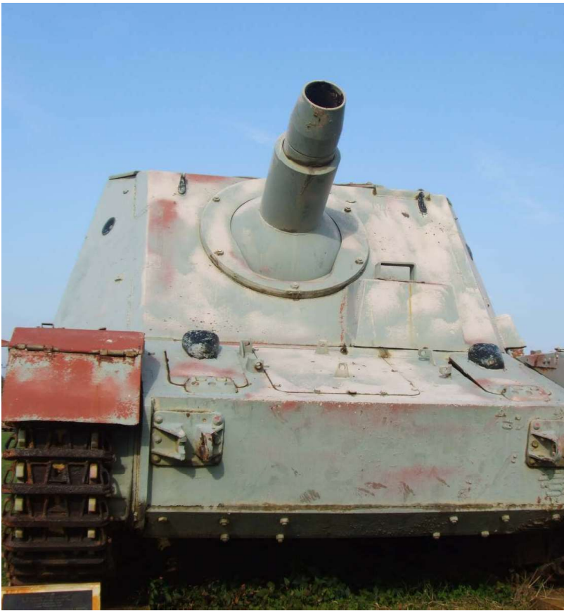
Sturmpanzers IV Brummbär (GERMANY): Mid-WWII Self Propelled Gun. Crew: 5. Main Armament: 150 mm. Machineguns: 1. Max Armor: 100 mm. Horsepower: 296 hp. Weight: 28.2 tons. Max Speed: 25 mph. Range: 130 miles. Number Produced: 306. Pros: Imposing, fully enclosed superstructure with up to 100 mm armor. Powerful infantry support 150 mm cannon. Cons: Not many other than slightly high profile, but even that was only 8' 3". Notes: The additional weight of the superstructure and cannon was too much for the Panzer IV chassis on which the vehicle was based. Later models had less armor and a redesigned, much lighter 15 cm L/12 cannon, which thus decreased strain on the suspension. This one was photographed at Aberdeen Proving Ground, Maryland.
