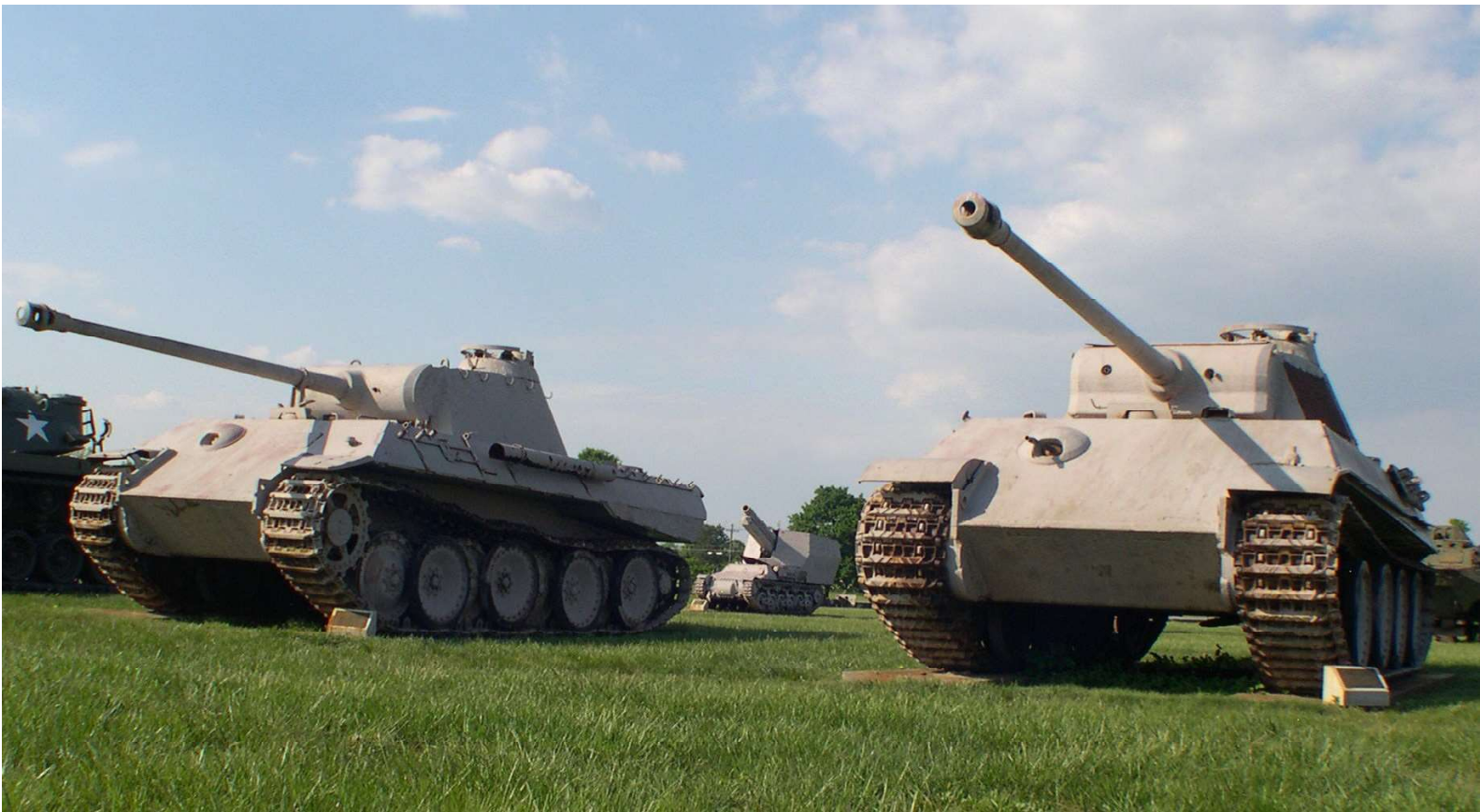
Panzer V (Panther) (GERMANY): Mid-WWII Tank. Crew: 5. Main Armament: 75 mm. Machineguns: 2. Armor: 16-110 mm. Horsepower: 690 hp. Weight: 44.8 tons. Max Speed: 34 mph. Range: 160 miles. Number Produced: 6,000. Pros: Well-balanced tank: hard-hitting, excellent thick, sloped armor and superb 75 mm main gun. Cons: Not many, but some complexity in the interleaved road wheel design. Notes: The Panther is perhaps the overall most well-balanced tank that the Germans made. It was inspired by the Soviet T-34. In fact, the Germans initially discussed simply making direct copies of the T-34, but national pride forbade that.
