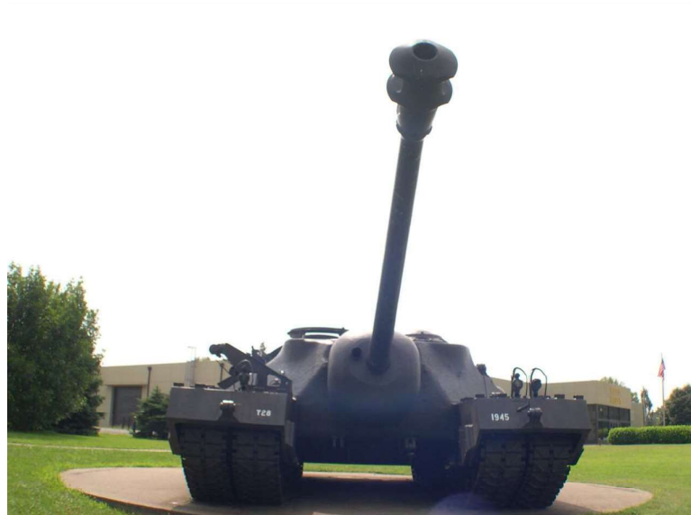
T28 (UNITED STATES): Late WWII Tank Destroyer. Crew: 8. Main Armament: 105 mm. Machineguns: 1. Max. Armor: 25-300 mm. Horsepower: 410 hp. Weight: 95 tons. Max Speed: 8 mph. Range: 100 miles. Number Produced: 2. Pros: Tremendous main gun and armor. Cons: Incredible weight. No turret. Notes: The T28 mounted a very powerful 105 mm anti-tank gun in a fixed superstructure. But instead of just one pair of tracks, the T28 had two tracks per side to handle the vehicle's massive weight. The outer tracks could be removed to allow the T28 to pass more easily in places and for easier transport. The dismantled tracks could be paired to each other and then towed by the T28 or by another vehicle. Only two were ever built; neither made it to combat, and one burned up in a fire.
