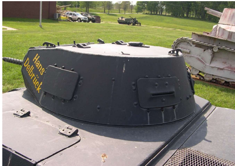
Panzer I (GERMANY): Tank. Produced: 1934-1938. Crew: 2. Main Armament: -. Machineguns: 2. Max Armor: 12 mm. Horsepower: 57 hp. Weight: 5.5 tons. Max Speed: 22 mph. Range: 125 miles. Qty. Produced: 2,000. Pros: Allowed the Germans to practice operating tanks. Cons: Too light for WWII combat. Notes: This tank was designed for training rather than real combat. Nonetheless, it saw extensive service in the battles for Poland, France and elsewhere. Its quick speed allowed it to help create havoc and confusion once it penetrated enemy lines. This vehicle was photographed at Aberdeen Proving Ground, Maryland.
